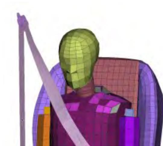
**Figure 5. A seatbelt going through a 3D slipping**
