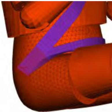
**Figure 4. Belt with 2D \*ELEMENT\_SEATBELT definition**
